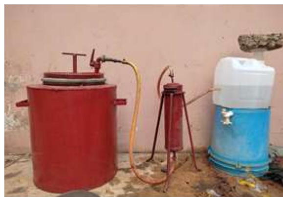
Plate 2: Field setup consisting of digester, purifier, storage tank and measuring cylinder
