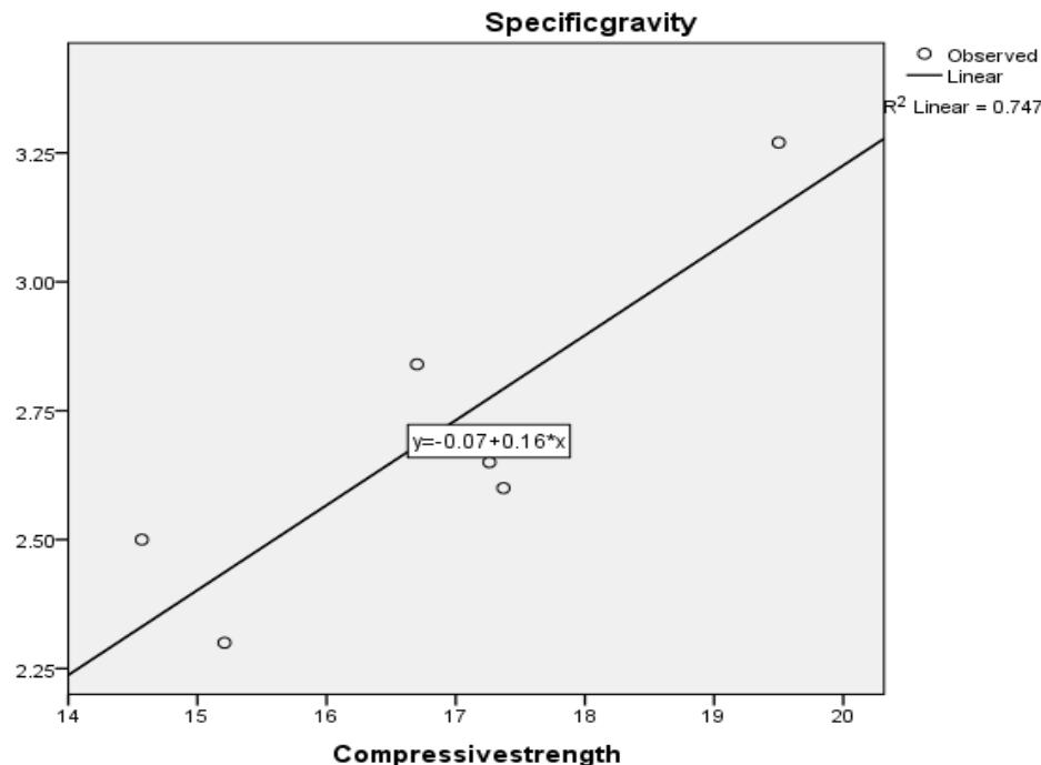
Figure 4. Graph of Regression Analysis of Compressive Strength against Specific Gravity
