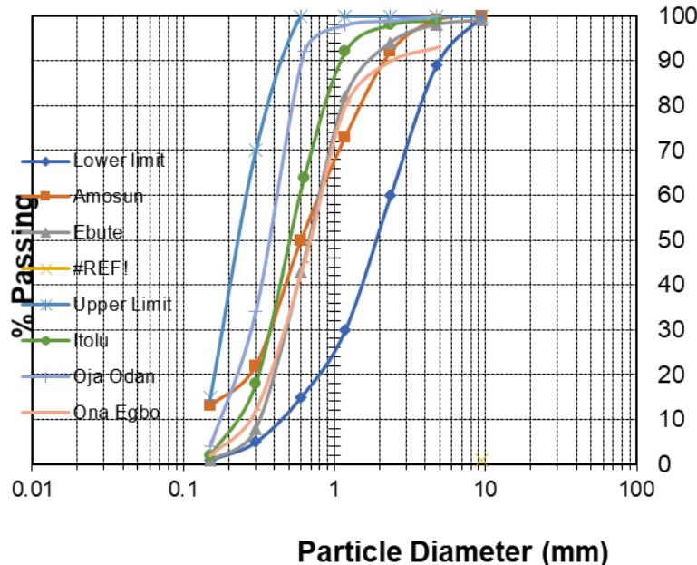
Figure 1 Sieve Analysis Graph of Samples from all locations
